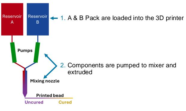
3. 3D printer moves position to create the desired part geometry4. Material reacts and begins to cure on the print bed
